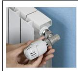
**3** - Position the thermostatic head onto the valve's body by centring the cap's hexagon and leaving the adjustment reference window upwards (in visible position).
