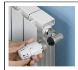
2 - Position the polymer spacer onto the valve's body by centring the cap's hexagon (this operation is necessary only for the 3087 series thermostatic head - the spacer is supplied as a kit with the thermostatic head).
